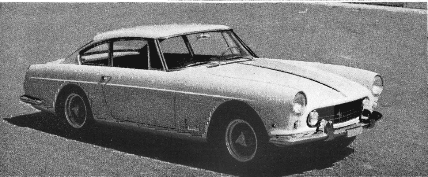
TOURING ELEGANCE.—The production Ferrari 2+2 which is developed directly from the 250GT, with 3-litre V12 engine, 4-seats and disc brakes. ↓
